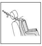
If the position you are using has an adjustable headrest or head restraint and you are using a single tether, raise the headrest or head restraint and route the tether under the headrest or head restraint and in between the headrest or head restraint posts.
